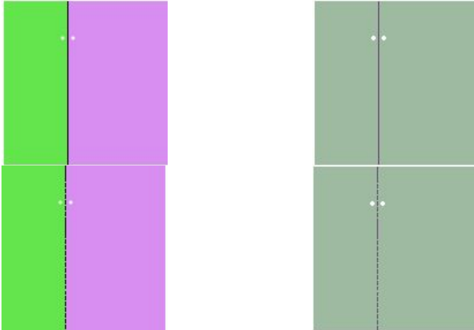
Figure 8: Errors in a Voronoi diagram using both the Cone algorithm (top) and the Tangent Plane algorithm (bottom). Images on right – 2 nd -nearest point diagram for 2 sites. Images on left – the corresponding 2 nd -order Voronoi diagram (containing just one cell). Black pixels in all images are erroneous. Note that the errors occur along the single boundary in the 2 nd -nearest point diagrams, thus in the interior of the resulting 2 nd -order Voronoi cell.
